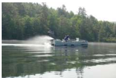
Figure 5: Pontoon boat utilizing an educator to disperse Renovate
