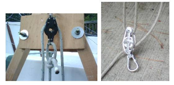
This block-wtih-becket makes the top half of a block and tackle. Other end is a fiddle block with becket. This end gets clipped to forestay tang with attachd shackle. See boat diagram on last page.
