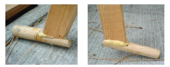
The feet are 1" dowels attached at an angle, so when the legs are spread so the feet are at the width of the handhold rails, they are perpendicular to the midline of the a-frame, like this:
