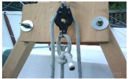
plywood sides glued to the 2x4, and the legs are bolted via pivot bolts to the plywood sides, allowing legs to open and close freely.
