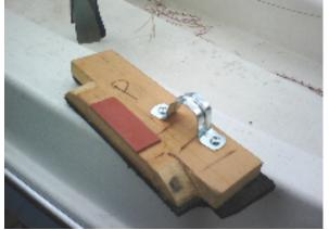
Made of 1x4 or something similar. Rubber pad is glued on the bottom, and a pipe hanger screwed to the top for the dowel to fit in. Note the rounded side extension - that fits under the teak handhold on the boat. I also use short straps wrapped around them and around the handhold rails so the bases won't tend to lift up or drift, but that's not totally necessary.
