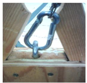
A screw eye is screwed into the spacer 2x4 at the top. A shackle is attached to the eye, and a swivel block with a becket is attached to the shackle. This eye is also used as attachment point for the line going to the jib halyard (see boat diagram on last page.)
