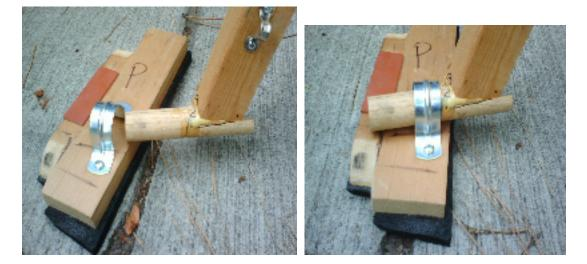
Above is a sequence of the foot fitting into the base
